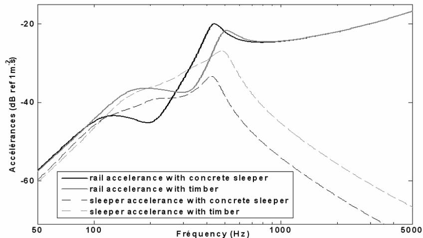
**Fig. 2.** Rail and sleeper accelerances, for concrete and wooden sleeper track. Track modelled with a Timoshenko beam continuously supported with a double stiffness layers: rail UIC60, ballast stiffness equal to 100MN/m<sup>2</sup>, railpad stiffness equal to 300 MN/m<sup>2</sup>, sleeper masses: concrete: 245kg timber: 96kg
