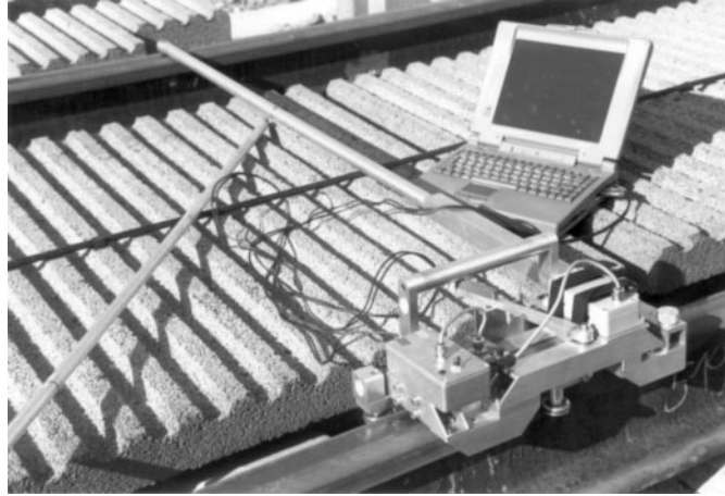
Figure 1. Corrugation analysis trolley.
