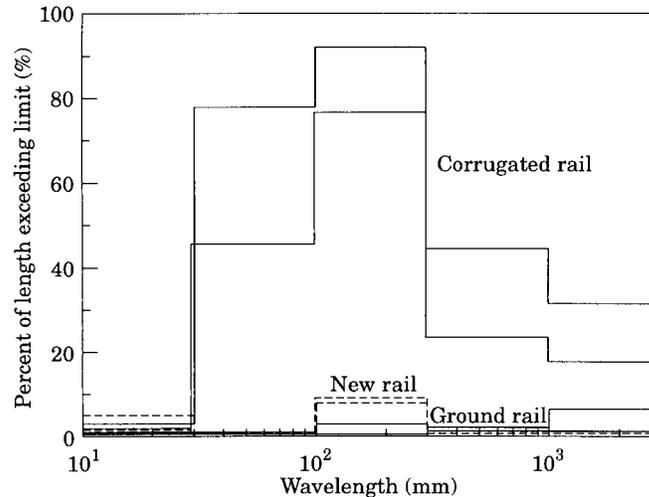
Figure 6. Fraction of rail exceeding amplitude limit.
