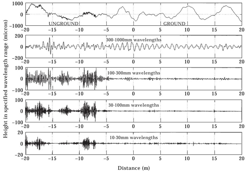
Figure 4. Overall profile of rail and wavelength components.
