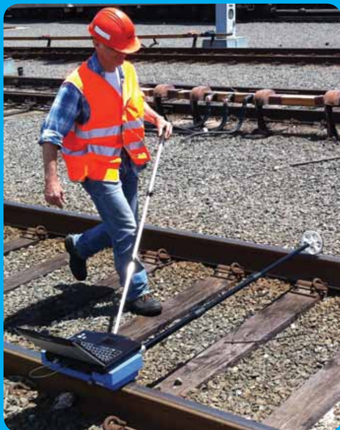
CAT in use. The equipment is suitable for both embedded and conventional flat-bottomed rails.
