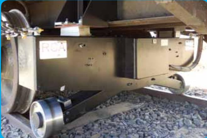
RCA fitted to chassis of the caboose on a main-line grinding train.
