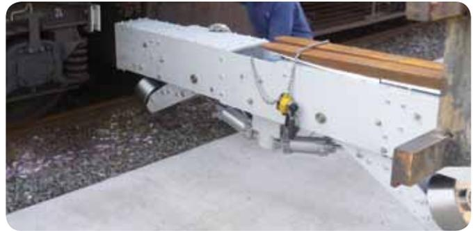
RCA being fitted to bogie of a reprofiling train using a forklift truck. Installation takes less than a day.
