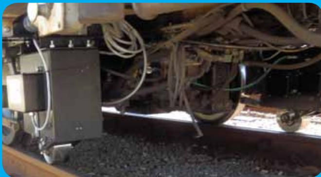
Gauge-adjustable RCA on a small metro grinder.
