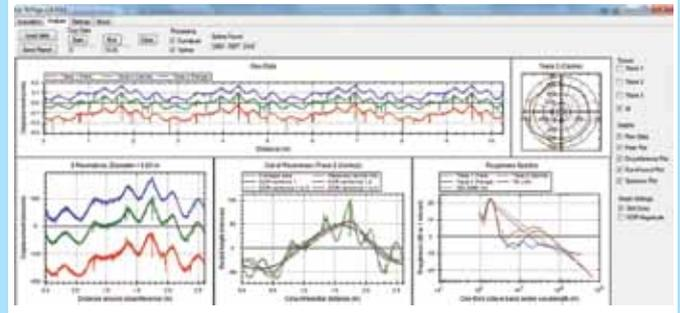
*Screen dump from a TriTops measurement of a wheel with out-of-round, a wheel flat of about 70µm depth (at about -155°) and a few smaller irregularities e.g. at -90°. Software shows that 3 full revolutions of the wheel have been made. The wheel diameter is calculated to be 0.83m. This analysis can be undertaken by clicking the appropriate tab and selecting a file as soon as a measurement is completed.*
