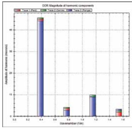
Out-of-roundness illustrated in two different ways. On the left, the harmonic components are summed and graphed as a function of circumferential distance. On the right, the harmonic components are shown. The fundamental harmonic at 0.35-0.4/m is indicative of a wheel that has worn with some eccentricity (about 46µm is suggested by the amplitude of the harmonic component). This is consistent with the "OOR harmonic 1" plot on the left.
