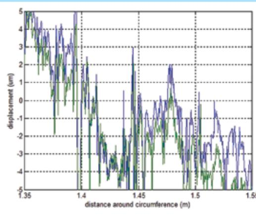
Demonstration of the repeatability of the TriTops. Two measurements are shown from consecutive rotations of the same wheel. On the left are the full records for the two rotations. On the right is a section of record expanded to a scale of +/- 5µm over 0.2m of the wheel.
