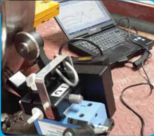
*TriTops in two configurations: attached to a rail (above) and to part of an underfloor wheel lathe (below). The instrument takes three measurements simultaneously around the periphery of a wheel. Data are logged to a laptop computer.*
