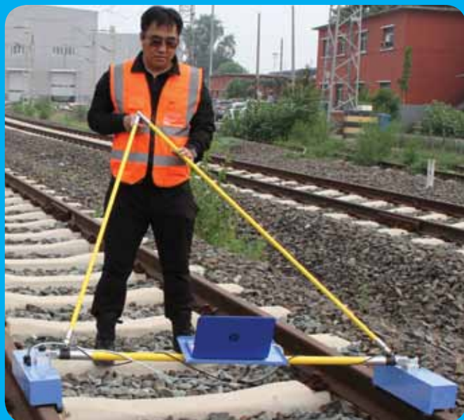
bi-CAT in use. The equipment is used by a single operator and is suitable for both conventional flat-bottomed and embedded rails.
